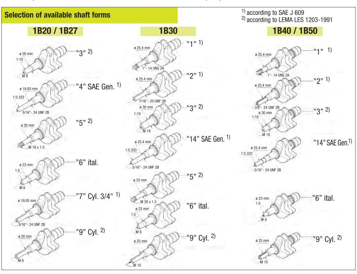
Drawings with detailed - and connection measures can either be demanded or downloaded as pdf- resp. dxf-file which are shown in the Internet.
