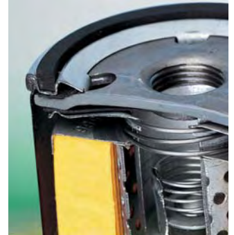
Cross-section of an oil filter
