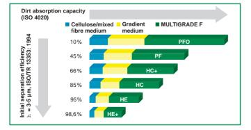
different performance characteristics, MANN+HUMMEL can provide fuel filtration systems which are perfectly matched to a specific application with regard to particle and water separation and service life MULTIGRADE F filter media consists of a combination of cellulose carrier medium and a melt-blown layer.
