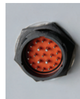
Pictured Above: Deutsch 21 pin engine harness connector
