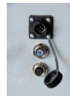
Top: CPC sealed dual float switch connector with cap Middle: M12 sealed transducer connector (cap not shown) Bottom: M12 sealed RS485 serial connector (cap not shown)
